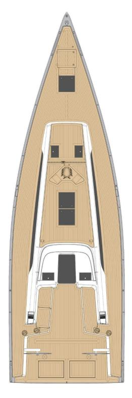
The standard layout plan offers a large sail locker in the bow with access through a flush hatch. In the stern, there are two flush hatches with storage, one for the gas bottles and the other for the life
